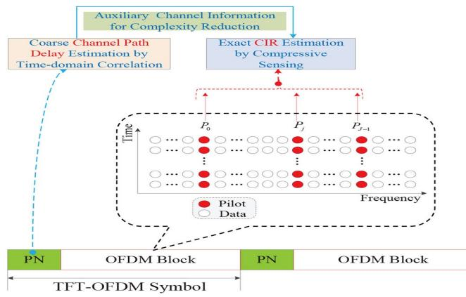
Figure 1: Proposed frame structure and the corresponding CS-based CE for the TFT-OFDM scheme.
