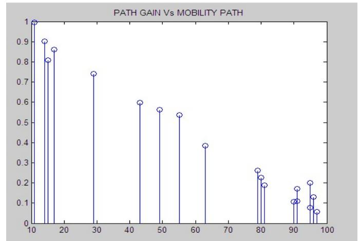
Figure 4: Channel path gains with a longer path delay
